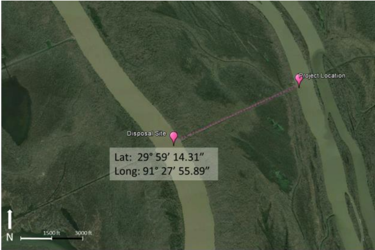
Figure 4: Location of disposal site. Dredged sediments will be deposited in the adjacent pipeline canal.
